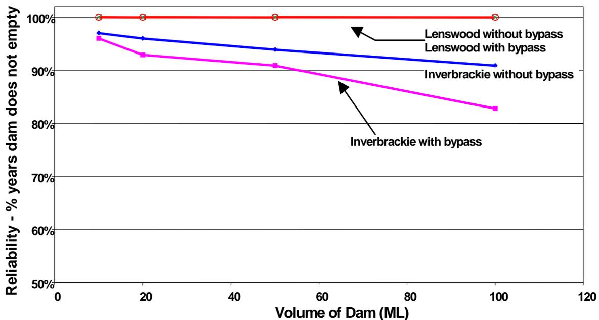
**Figure 5.** Effect of low flow bypasses on reliability of farm dams.
