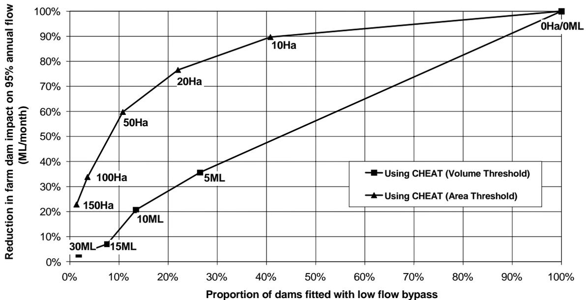
**Figure 4.** Reduction in impact on low flows for farm dams with low flow bypasses installed, using volume or area thresholds for selection.
