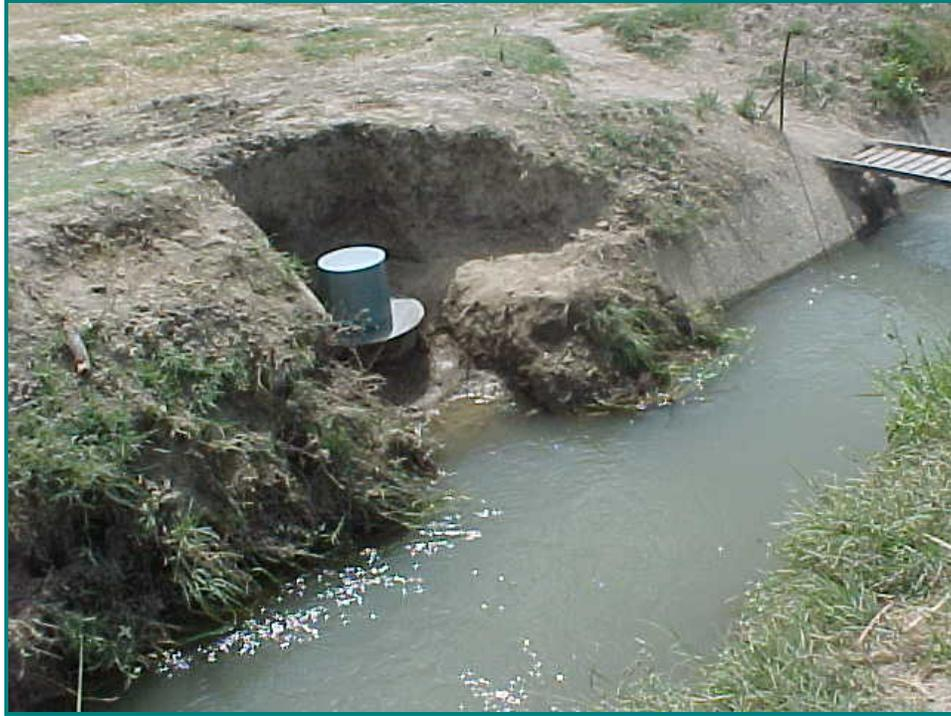
**Picture 3. Sensor installed on intake “Fixed channel”**
