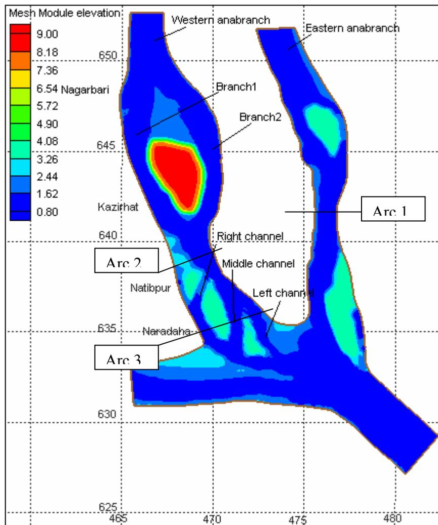
Fig. 4.1 Initial bathymetry in April 2001
