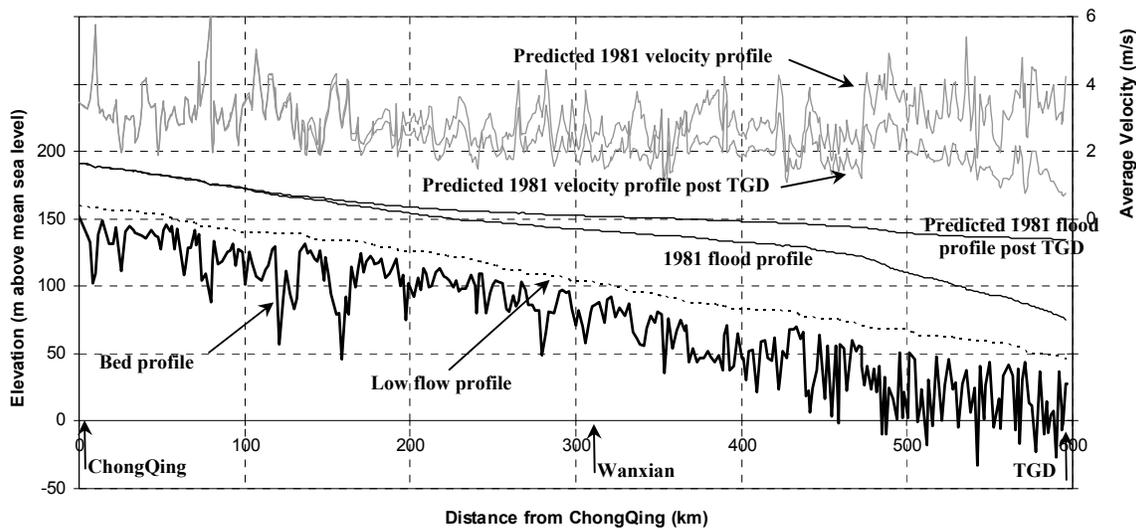
**Figure 2.** Long section of predicted water surface profiles associated with low flow conditions and the 1981 flood event through the upper reach of the Yangtze River under pre and post Three Gorges Dam conditions
