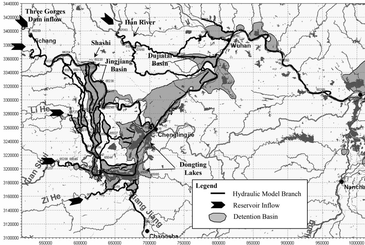
**Figure 3.** Middle Reach of the Yangtze River with Hydraulic Model Layout Superimposed.
