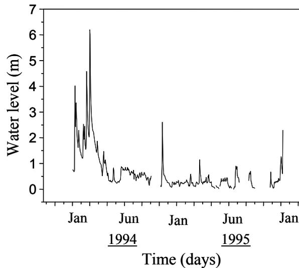
Figure 2: Stage evolution at Belksiri hydrological station during 1994 and 1995
