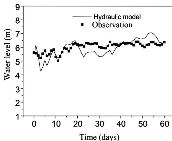
Figure 4: Calibration of the hydraulic model, the Lalla Aicha dam, Jun-July 1997
