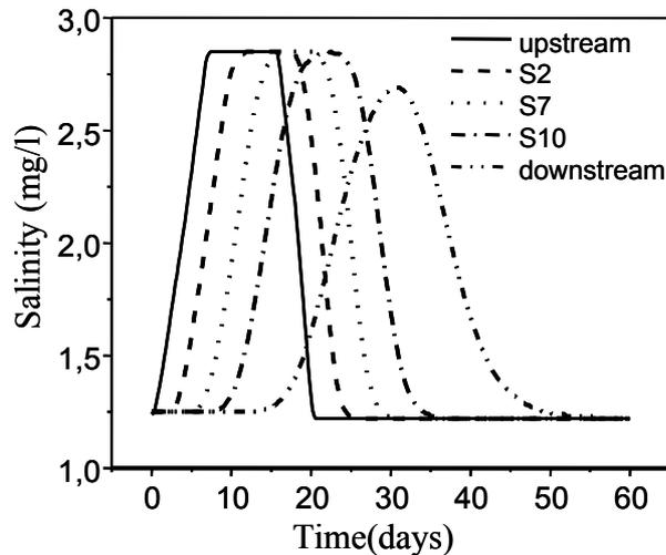
Figure 7: Evolution of a salinity intrusion at different stations for a  $25 \text{ m}^3 \text{ s}^{-1}$
