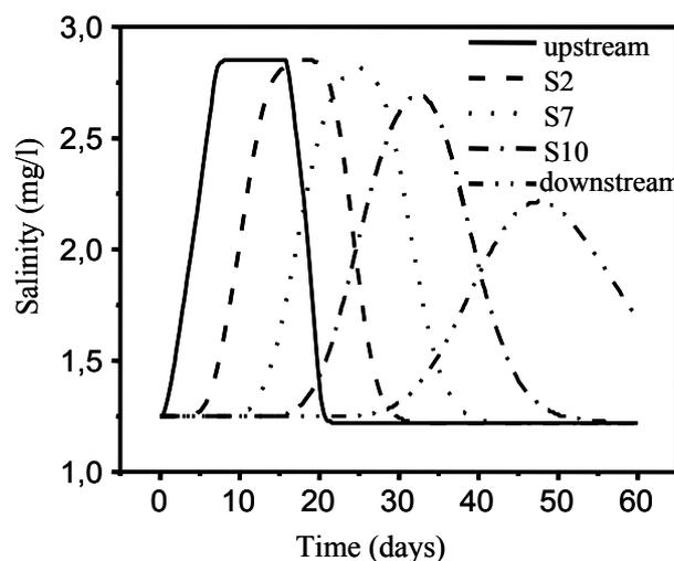
Figure 6: Evolution of a salinity intrusion at different stations for a  $10 \text{ m}^3 \text{ s}^{-1}$
