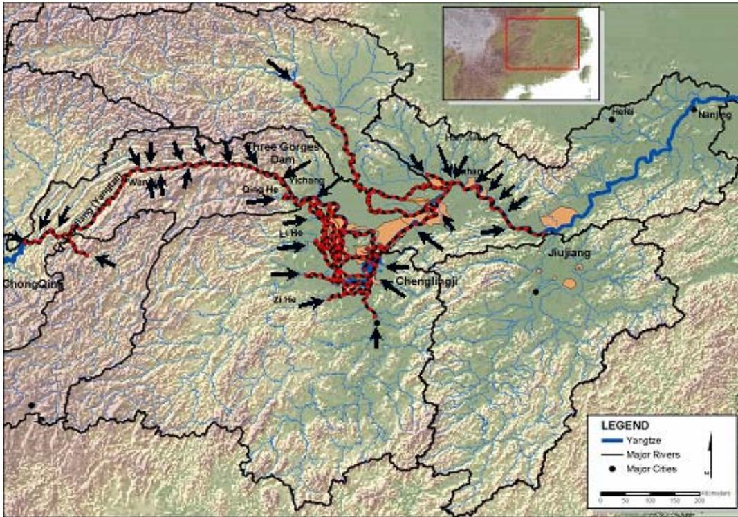
**Figure 3.** Linkage of hydrologic (tributary inflows) and hydraulic (main stem) models in the FFS
