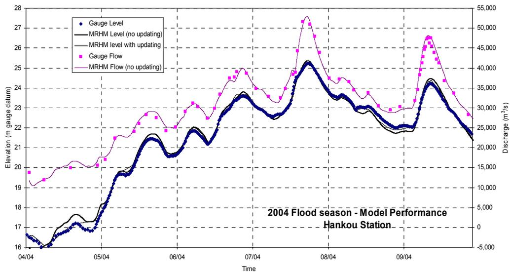
**Figure 5.** Comparison between the predicted and observed water levels and discharges at Wuhan (Hankou) for the 2004 flood season (MRHM – Middle Reach Hydraulic Model)
