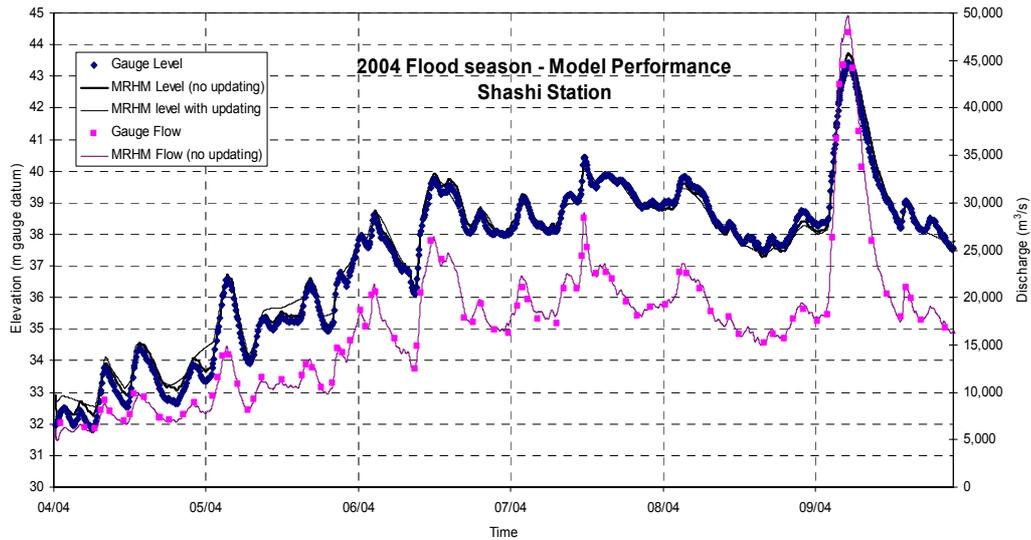
**Figure 4.** Comparison between the predicted and observed water levels and discharges at Shashi for the 2004 flood season (MRHM – Middle Reach Hydraulic Model)
