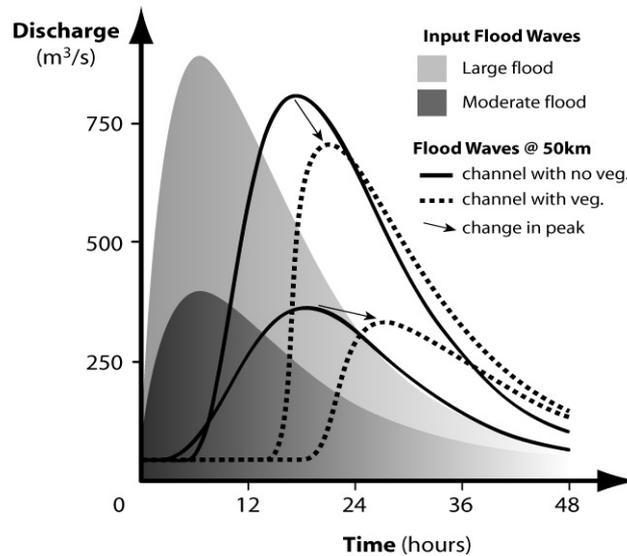
Figure 3 Numerical routing of two flood waves down a 50 km reach, with and without vegetation.
