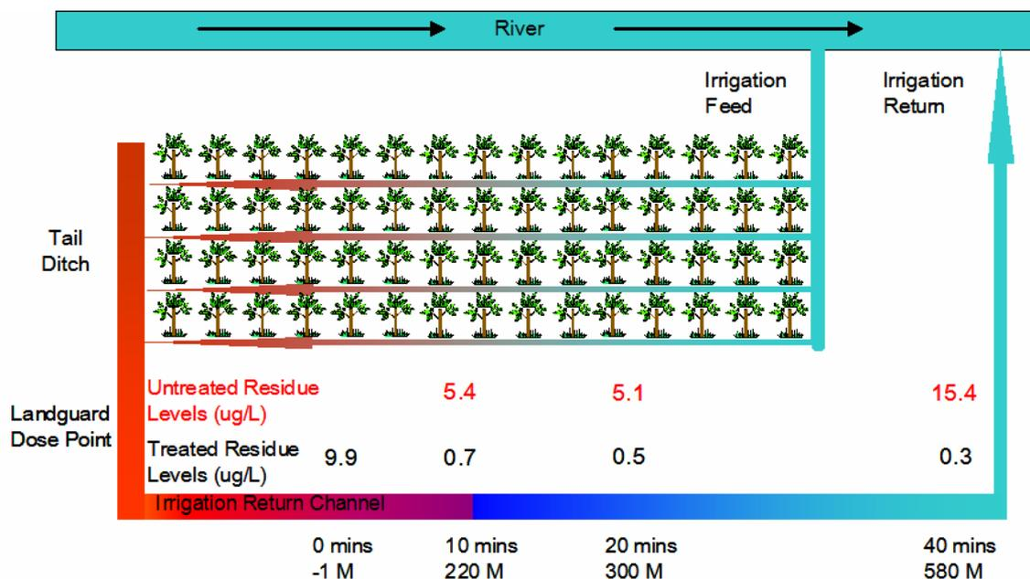
**Figure 9: Layout of the cotton farm and m-parathion residue levels observed pre and post treatment.**
