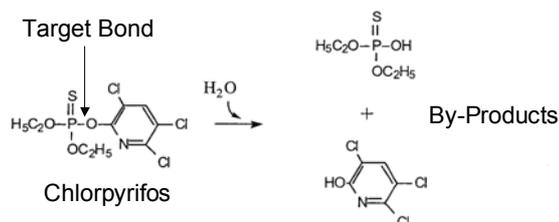
Figure 2. Chlorpyrifos hydrolysis reaction.
