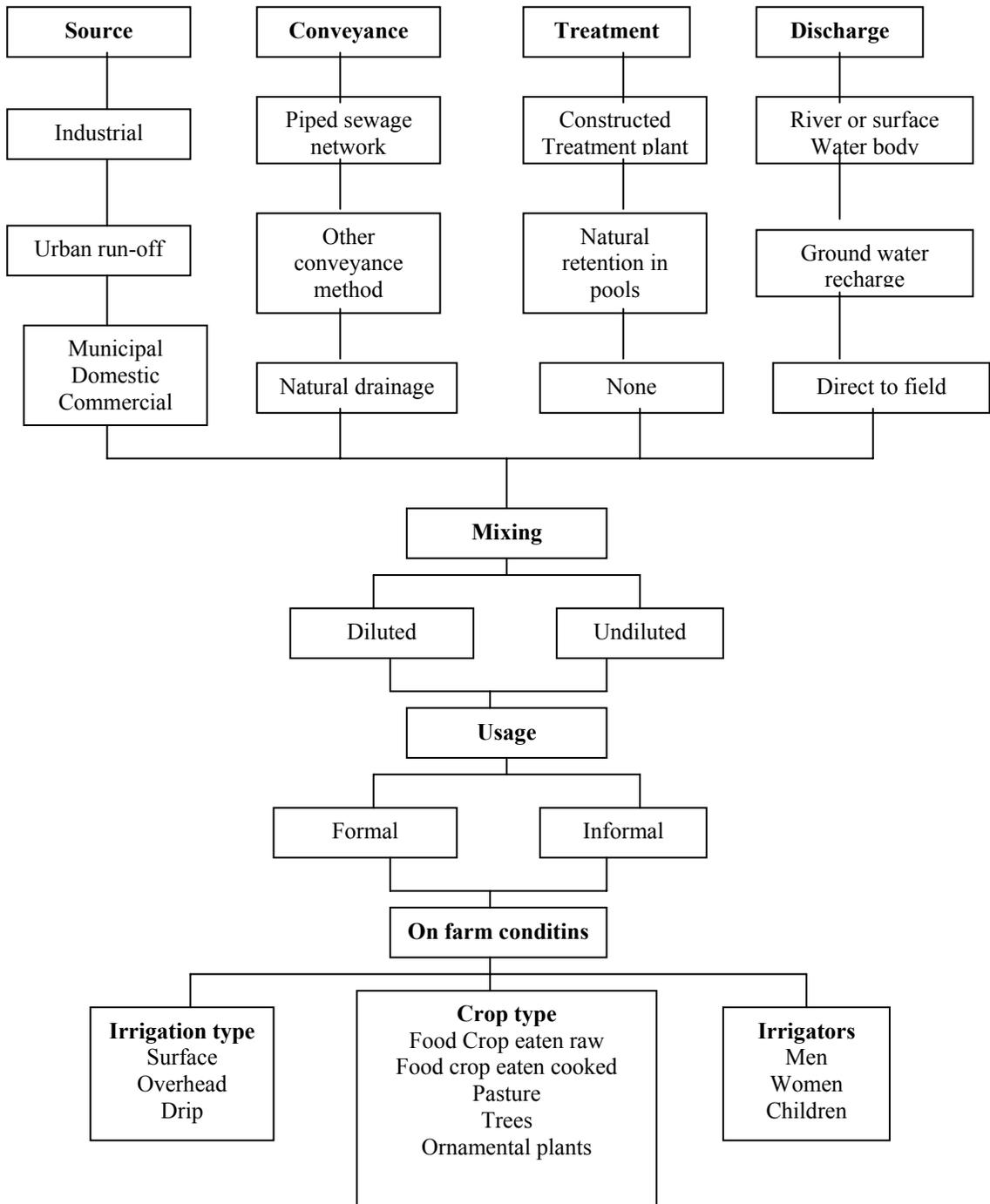
Figure III Typology of wastewater irrigation (Source : Buechlar, 2002)
