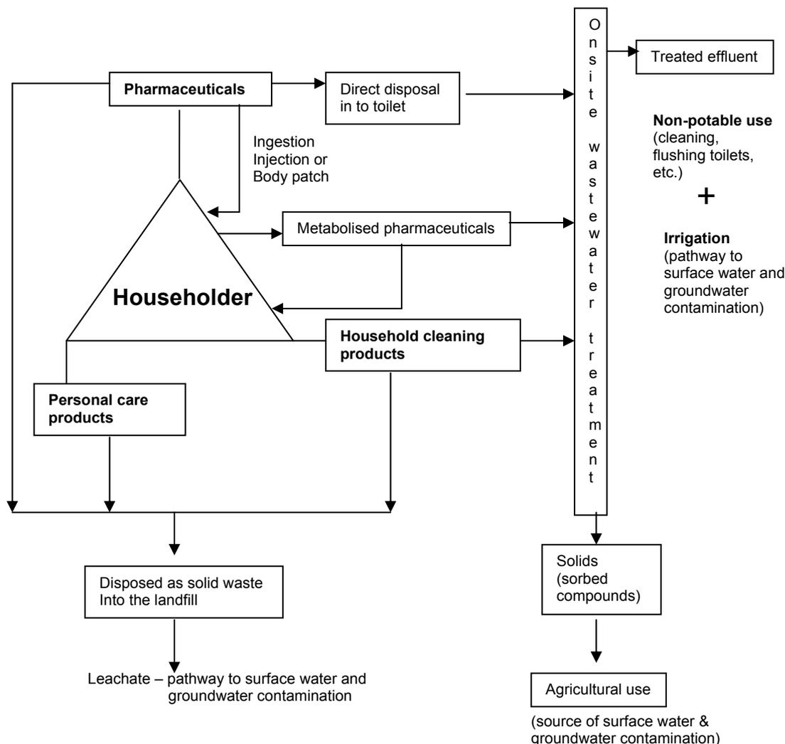
Figure: 2 Fate and possible pathway of compounds disposed in domestic wastewater
