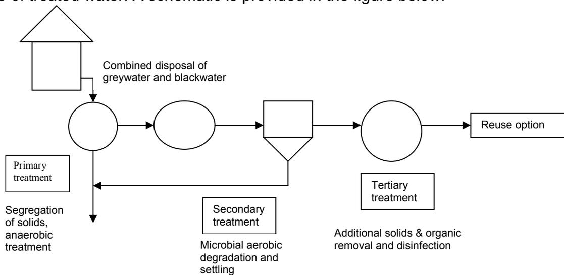
Figure 1. Schematic of a treatment processes in an on-site wastewater treatment system
