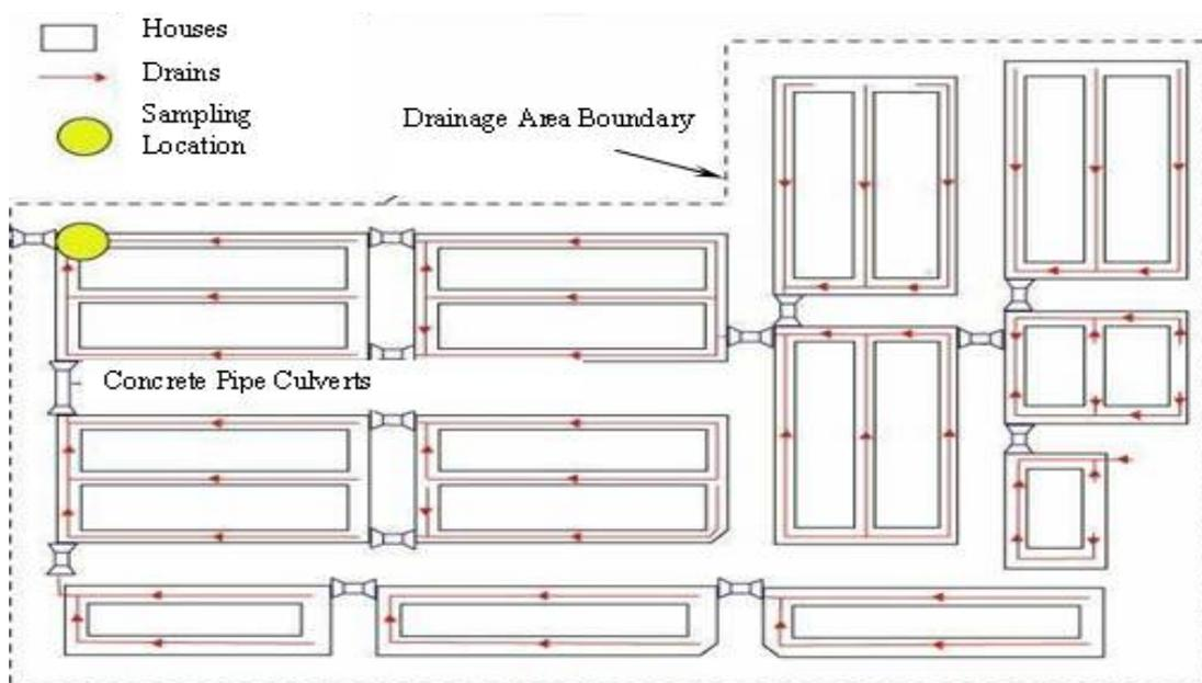
Figure 1. Schematic of the drainage system (not to scale)
