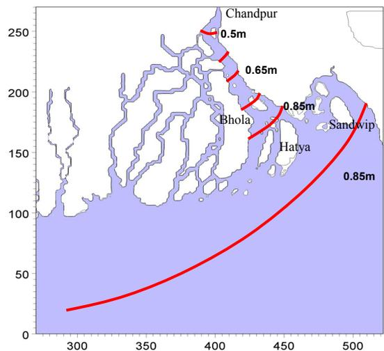
**Figure 3.** Rise of water level due to 88 cm SLR
