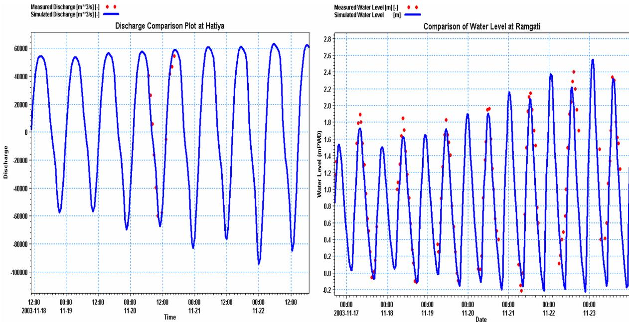
**Figure 2.** Calibration of the model against flow and water level
