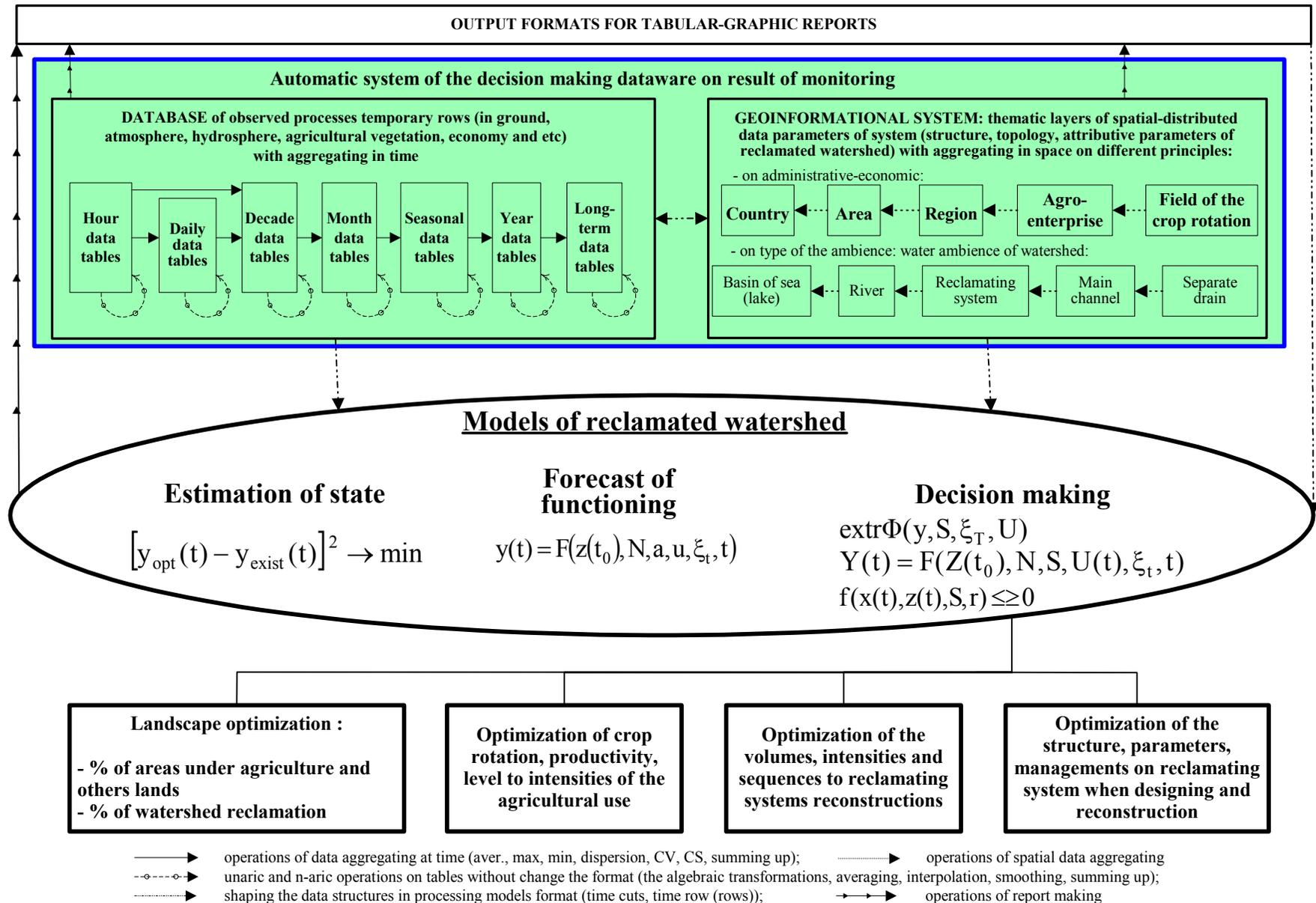
**Fig. 2. Information system of spatial-temporal monitoring for estimation, forecast and decision making on reclaimed river watersheds**
