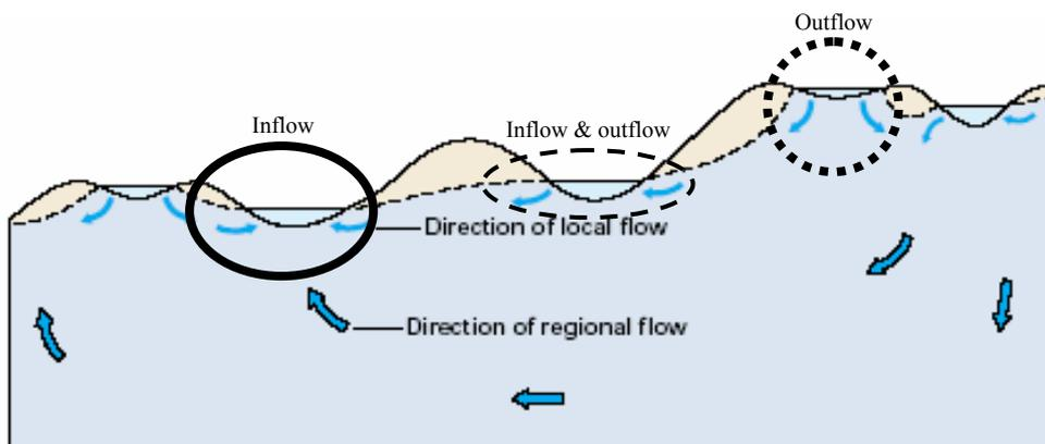
**Figure 3.** Schematic of on-farm dam surface-ground water interactions (Winter *et al*, 1998).
