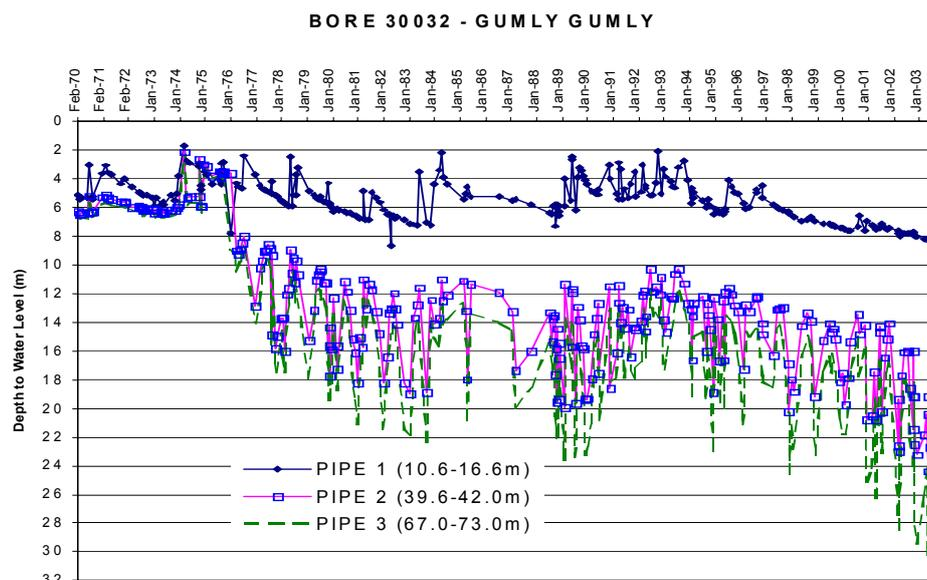
**Figure 7.** Groundwater Response Close to Gumly Gumly Borefield.
