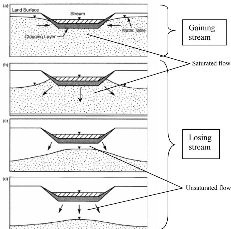
**Figure 2.** Schematic representation of influent and effluent streams (Peterson and Wilson, 1988). (a) represents a connected gaining stream, (b) represents a connected losing stream, (c) represents a disconnected stream with a shallow aquifer and (d) represents a disconnected stream with a deep aquifer.
