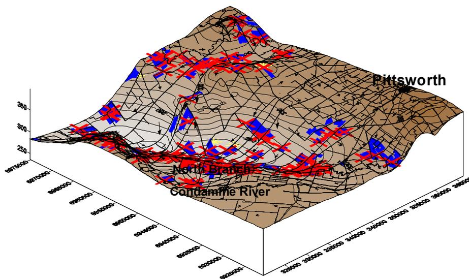
Figure 5. Shape of bedrock of the Condamine aquifer.
