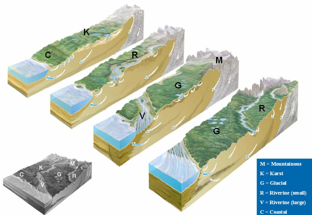
**Figure 1.** Schematic representation of the 5 main surface-ground water interactions (Winter *et al*, 1998).
