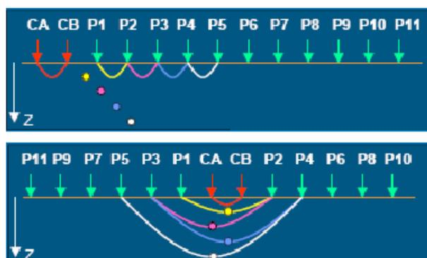
**Figure 9.** Diagram of the Dipole-Dipole and Wenner-Schlumberger arrays.
