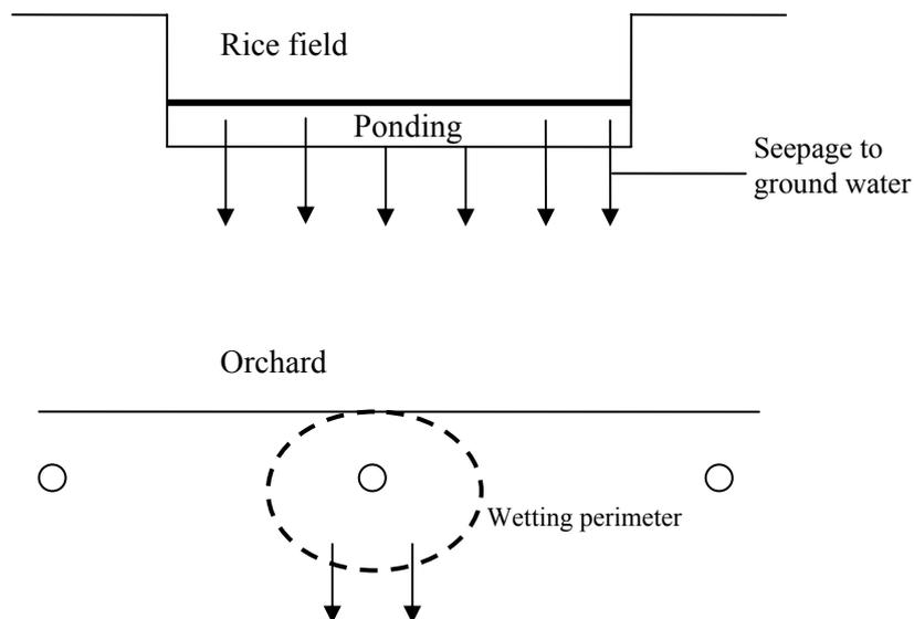
**Figure 4.** Schematic representation of the seepage from different types of irrigation methods.
