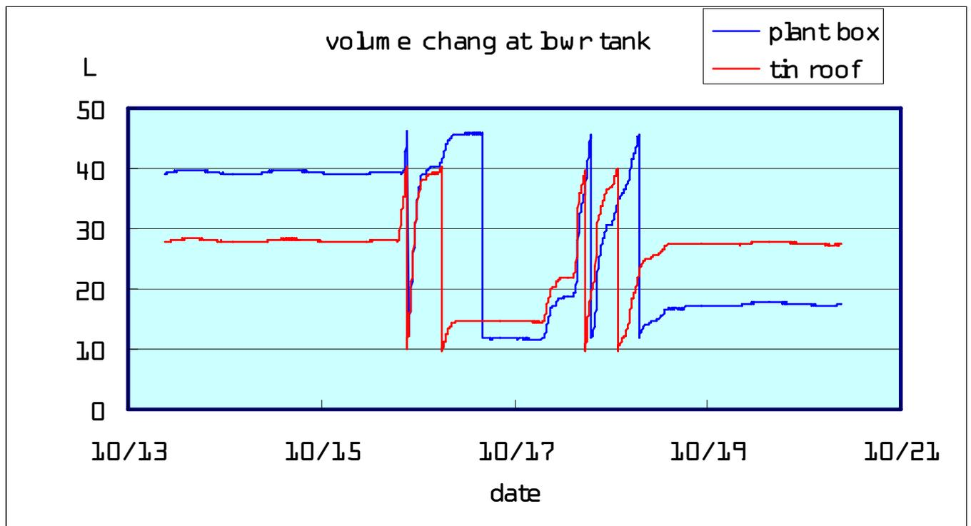
Figure 4 Record of water level change in lower tank
