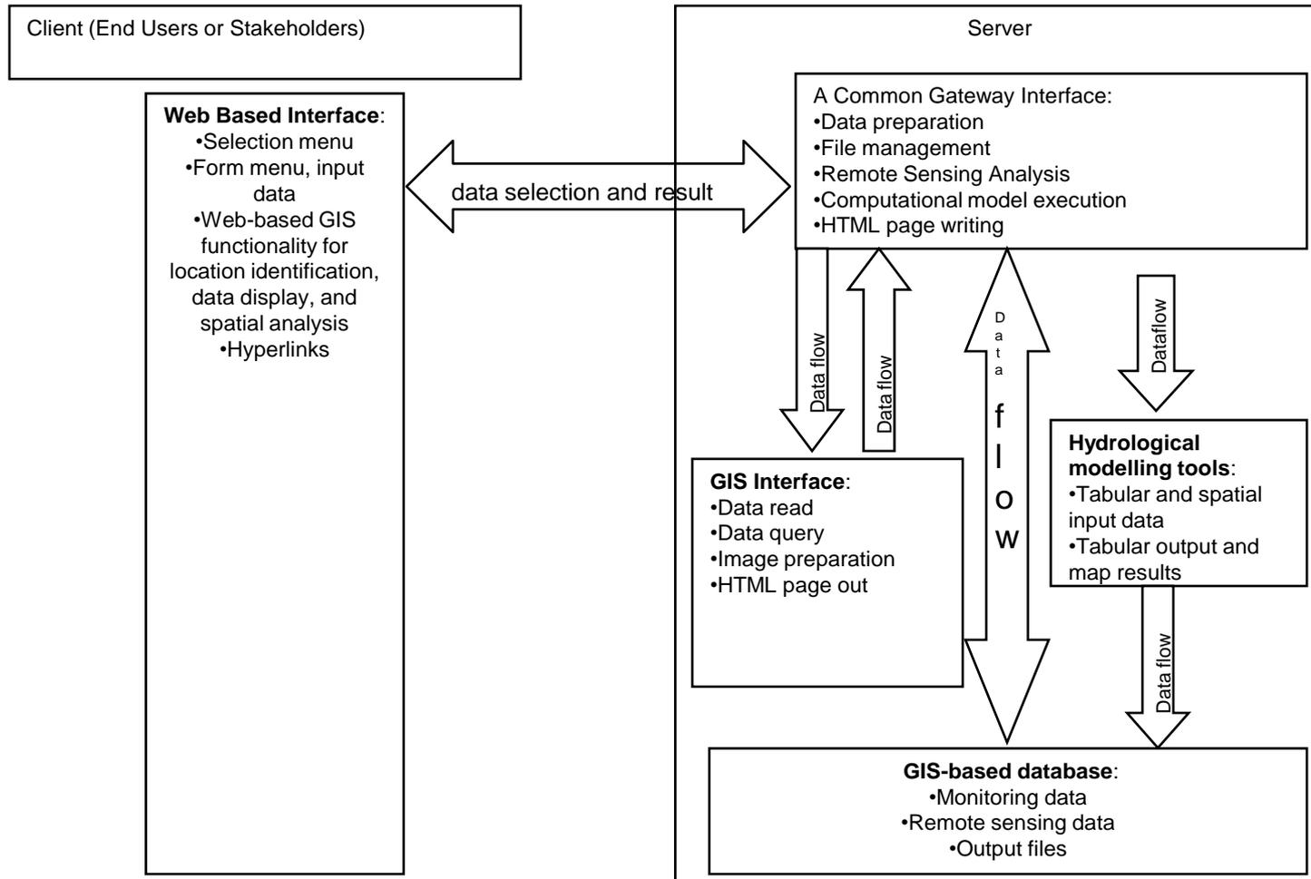
Figure 1. Schematic diagram of a hydroinformatics system for an irrigation district.
