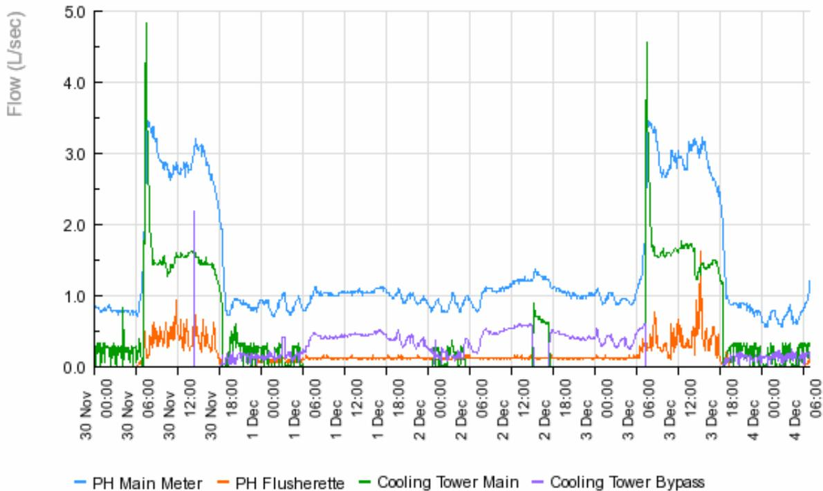
**Figure 3: Monitoring data of the main, cooling tower and flusherette water meters.**
