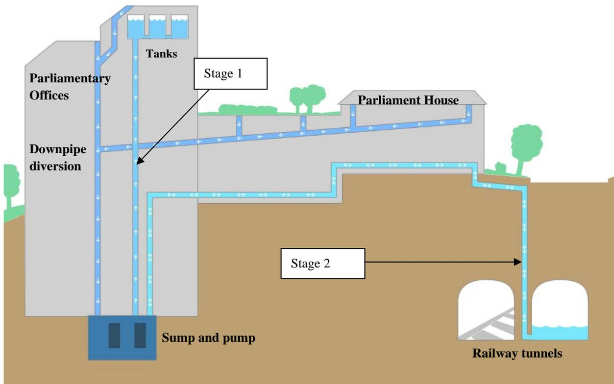
**Figure 4: Layout of the water collection and re-use system**
