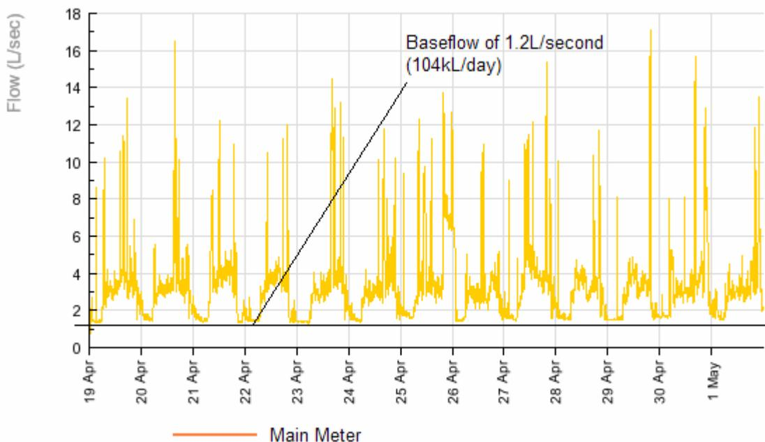
**Figure 8: Main meter water usage profile showing 1.2L/second baseflow**
