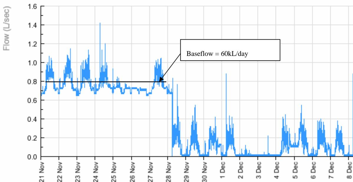
**Figure 1: Monitored water usage profile in an office building showing baseflow repair**
