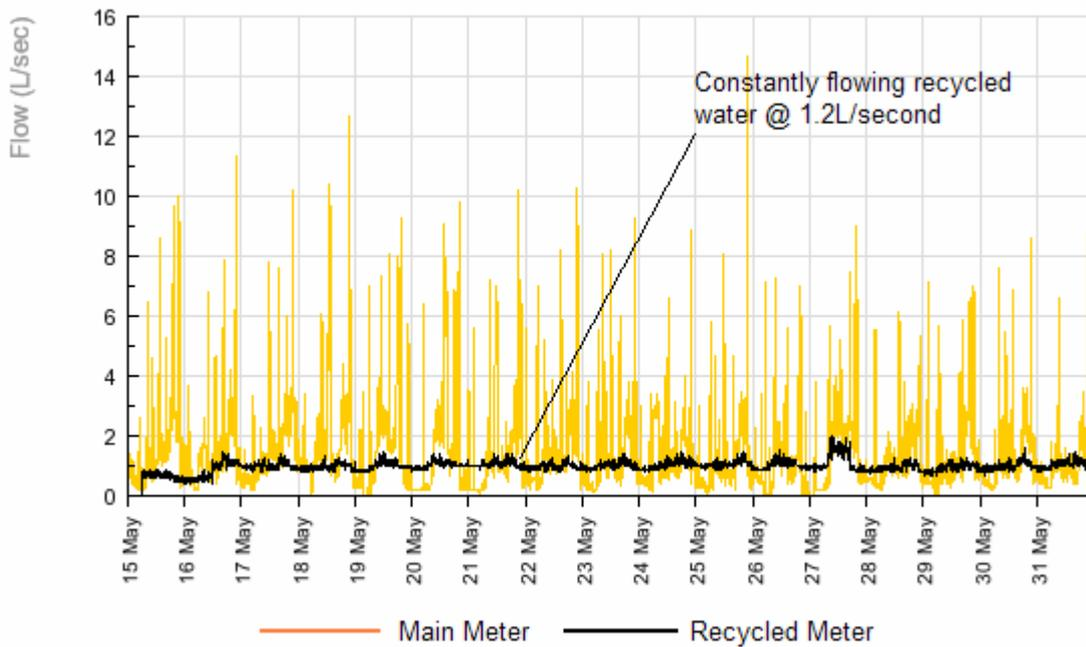
**Figure 9: Main meter and recycled water meter usage profiles showing baseflow transferred to recycled water**
