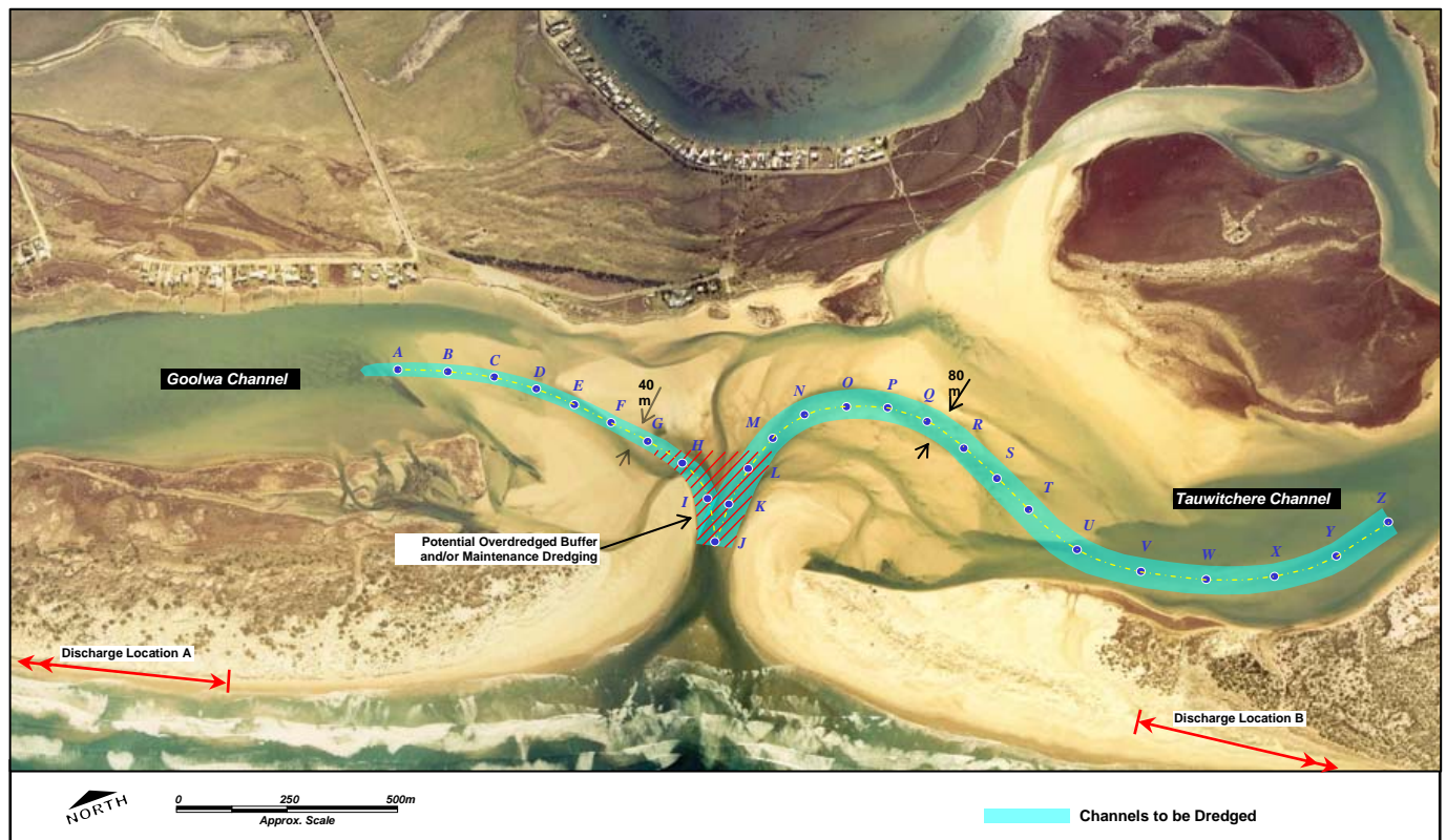
Fig 2. Engineered channels (Source: BMT WBM)
