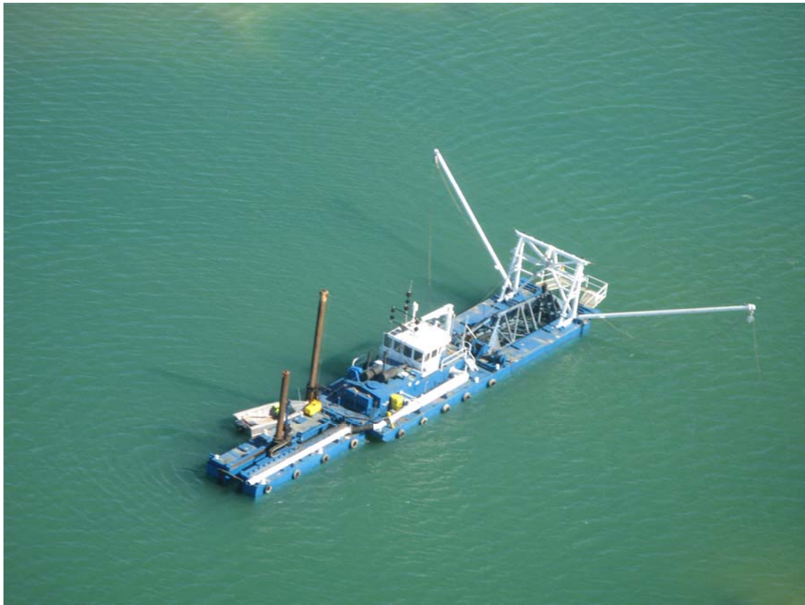
Fig 3. Cutter Suction Dredge currently operating at Murray Mouth (Source: DWLBC)
