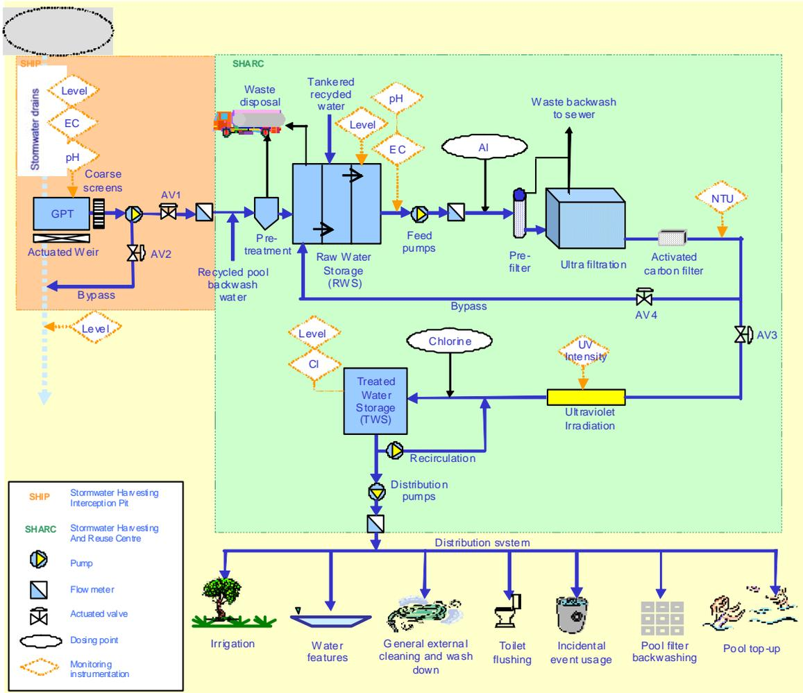
Figure 2 South Bank SHARC Flow Schematic
