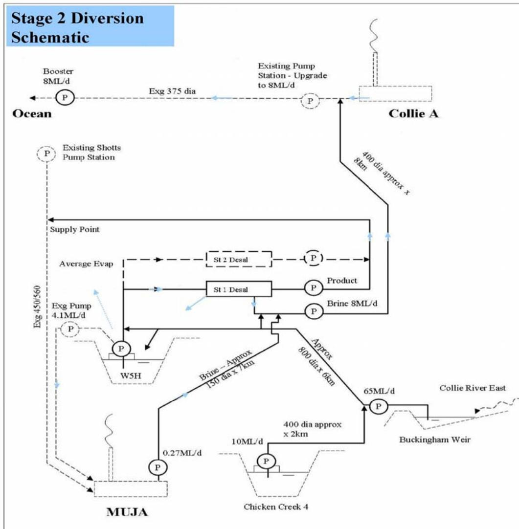
Figure 6 Schematic of Stage 2 Diversion Infrastructure
