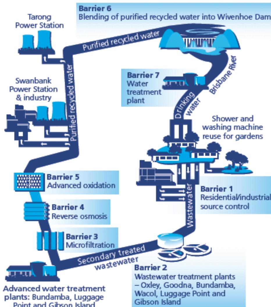
The Western Corridor Recycled Water Project provides three barriers in this process, microfiltration, reverse osmosis and advanced oxidation, through its advanced water treatment plants.
